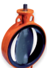
Series 75/31 Semi-lug butterfly valve, centric with fixed liner DN50-300 PN10/16 Ductile iron
