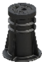
Series 80/32 Surface box "Futura" for service connection valves Fixed height Body of PA+ Lid of yellow PA Options: • lid of cast iron or black PA • for pavement
