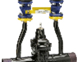
Series 46/80 Gate valve with long spigot ends and two purge points DN80-600 PN16 GP240GH With external PUR coating
