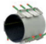
Series 748/03 Repair clamp Triple band with support plate Stainless steel AISI 304 or AISI 316 NBR or EPDM rubber Options: • fingers
