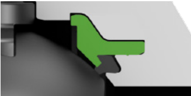
(4) The seat retainer design ensures the ball seat is kept in place. It prevents the ball seat from being dislodged, which guarantees a good functionality throughout the years.
