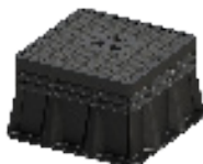
Series 80/36 Surface box for gate valves to DIN 3583 Fixed height Body of PA+ Lid of cast iron Options: • height adjustable • synthetic lid • to DIN 3584
