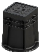
Series 80/34-000 Surface box for gate valves to DIN 3581 Fixed height Body of PA+ Lid of cast iron
