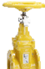
Series 06/59 Flanged gate valve with position indicator Short DIN F4 DN50-400 PN10/16 Ductile iron With external epoxy coating
