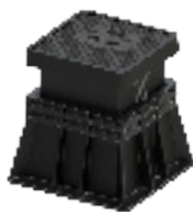
Series 80/35 Surface box for gate valves to DIN 3582 Height adjustable Body of PA+ Lid of cast iron Options: • fixed height
