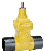
Series 46/64 Gate valve with short spigot ends DN50-300 PN16 GP240GH With external epoxy coating
