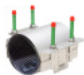
Series 748/02 Repair clamp Single band with support plate Stainless steel AISI 304 or AISI 316 NBR rubber Options: • fingers • handgrip
