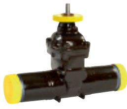
Series 46/78 Gate valve with long spigot ends and ISO top flange DN50-400 PN16 GP240GH With external PUR coating
