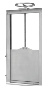
Series 772/7172 Channel penstock Uni-directional up to and incl. 1000 x 1000 mm, bi-directional in larger sizes With non-rising stem Stainless steel AISI 304 200 x 200 mm - 2000 x 2000 mm
