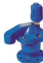
Series 701/50 Combination air valve Inlet flange DN50-300 PN16 Grey cast iron/Reinforced polyamide
