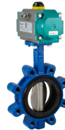
Series 820/10 Butterfly valve Centric with loose liner Lug type DN25-600 PN10/16 Ductile iron
