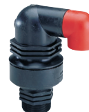
Series 701/40 Combination air valve DN20, 25 and 50 Threaded BSP ¾", 1" or 2" PN16 Reinforced polyamide
